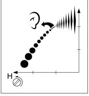
The high speed needle H is correctly set when the saw "4-cycles" a little. If the saw "whistles" the setting is too lean. If there is too much exhaust gas at the same time as the saw "4-cycles" much, the setting is too rich. Turn the high speed needle H until the setting sounds correct. NOTE! For optimum setting of the carburetor, contact a qualified servicing dealer who has a revolution counter at his disposal.
